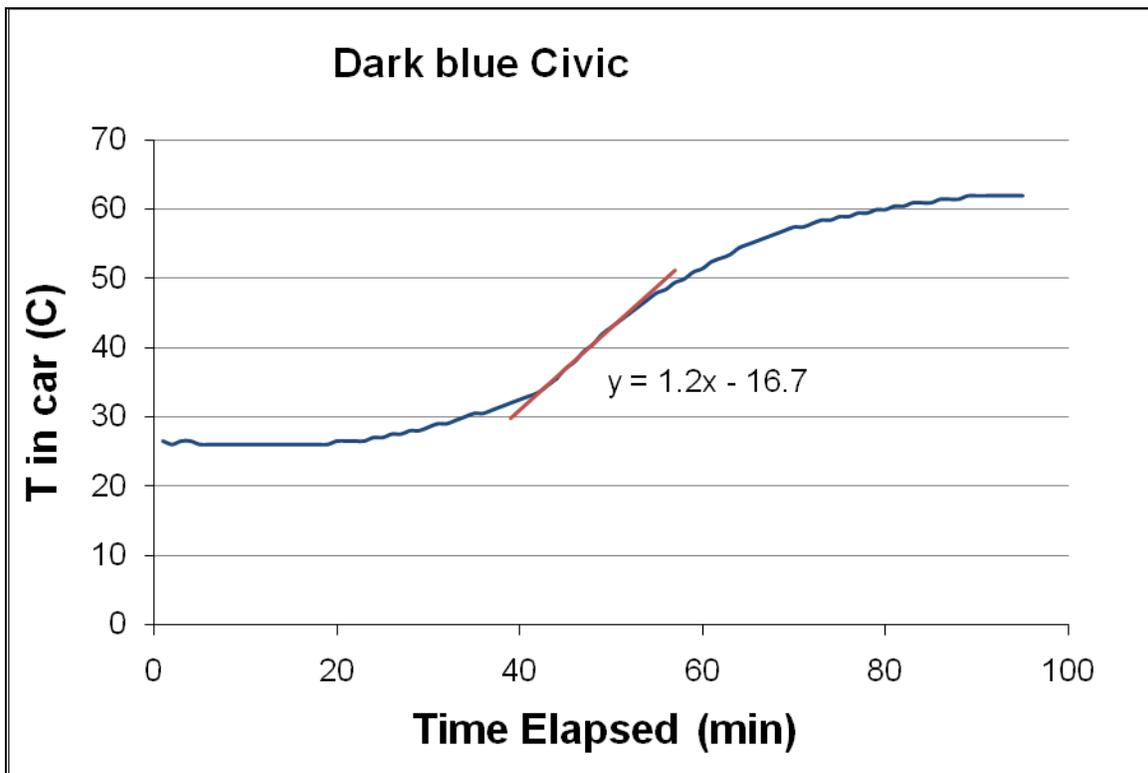
**Figure 1.** The heating of a dark blue Honda Civic – when left in the sun on a hot day, the car heated up at a rate of  $1.2^{\circ}\text{C}/\text{min}$  to a final temperature of  $62^{\circ}\text{C}$ .
