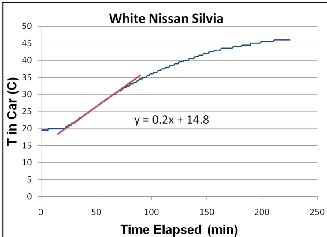
**Figure 2. The heating of a white Nissan Silvia** – when left in the sun on a hot day, the car heated up at a rate of 0.2°C/min to a final temperature of 46°C.
